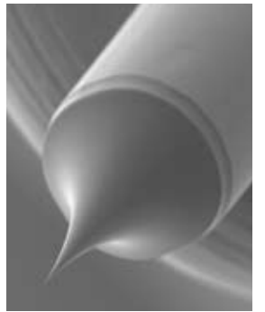
Cold field emission tip
