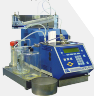
Noack - Evaporation Loss
